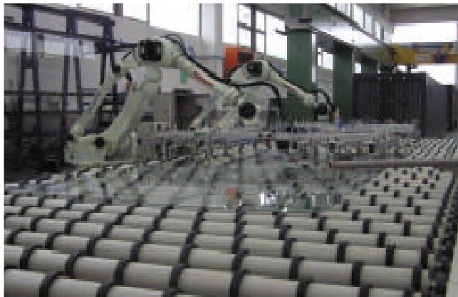
Two synchronized seven axis industrial heavy payload robots.
