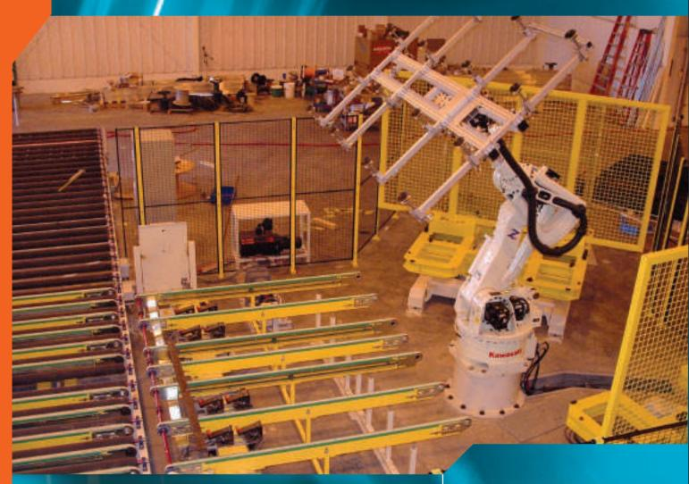
I-Scan has developed new robotic cells which allow loading as well as unloading operations of various glass sizes, from split to LES, providing an automatic flexible solution for tin side/air side handling.
