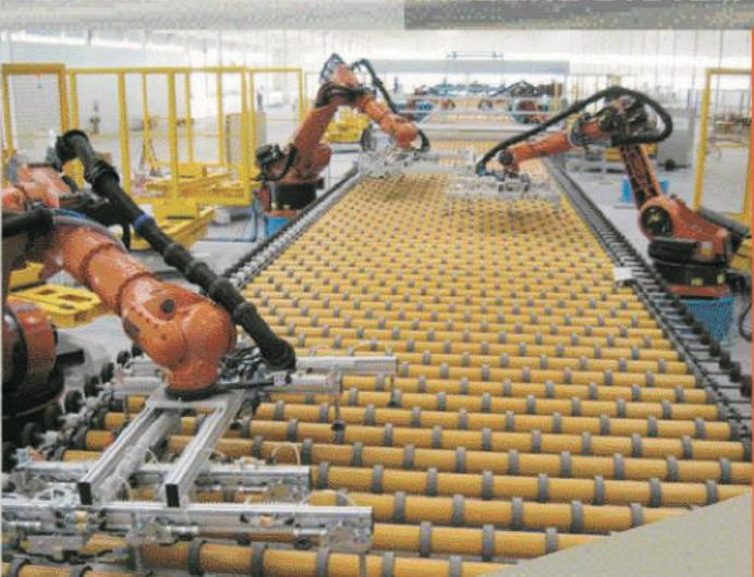
The Hawk is a highly versatile and comprehensive "state-of-the-art" robotic workcell for optimal unloading of flat-glass plates directly off a running float line. By using this amazingly flexible and modular glass handling system, flat-glass manufacturers achieve higher quality levels, increase throughput, minimize damage and reduce operating costs.
