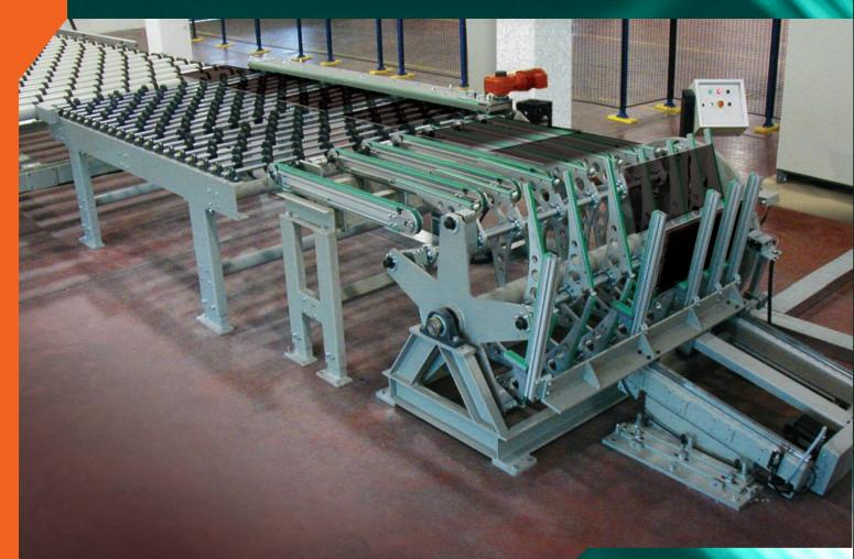
The Falcon is an exceptional swift automatic system for stacking small glass plates. This ultra-fast system can reach a stacking cycle of 1.1 second per plate and is built for handling small splits, from 4 plates up to 10 or 12 plates across the ribbon.
